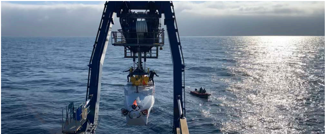
The two swimmers on top of Alvin remove the deployment rope once the sub is in the water and are then picked up by the small, motorized boat, which is waiting in the back. Photo credit: Tina Treude
